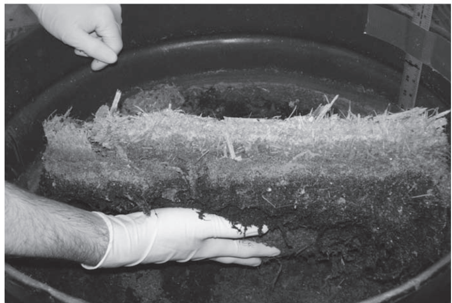
Figure 1. Picture of a portion of the spoiled material removed from an open barrel. Layers of moisture loss, mold, and decomposition can be seen.
