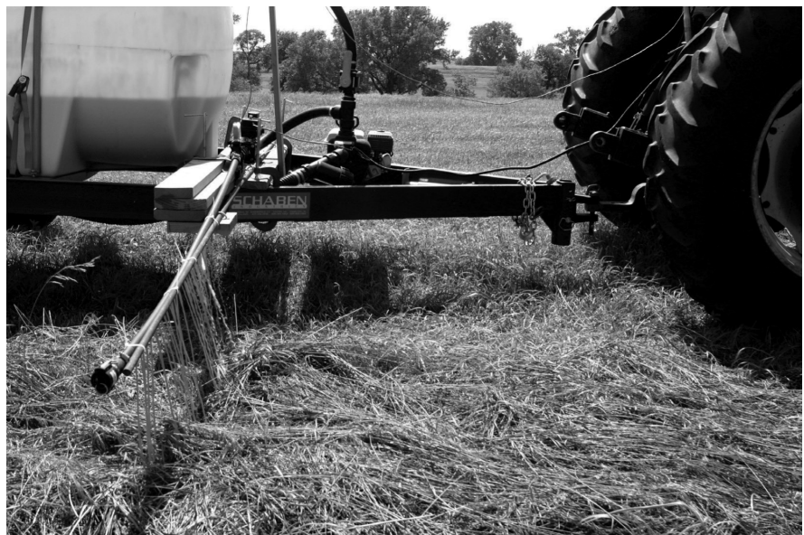
Figure 1. Liquid trailer with modifications to apply CCDS to hay windrows.
